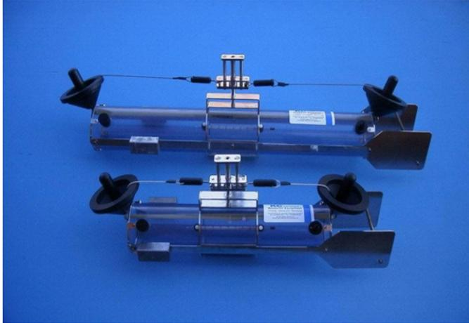
**Gambar 6.3:** Alat Sampel Air Horizontal
